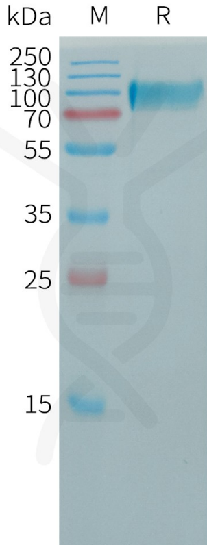
Figure 1. Human BCHE Protein, His Tag on SDS-PAGE under reducing condition.
