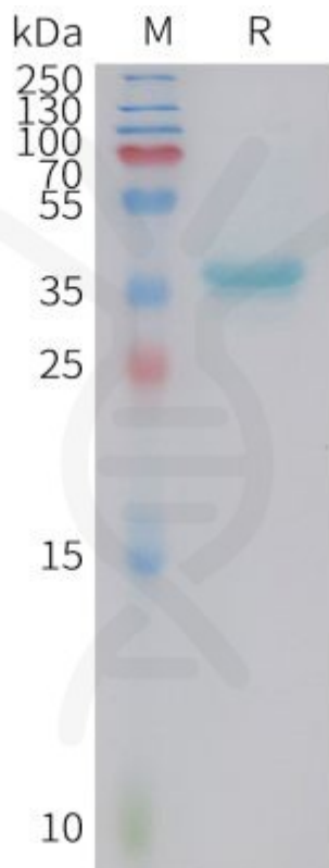
Figure 1. Human GAL Protein, hFc Tag on SDS-PAGE under reducing condition.
